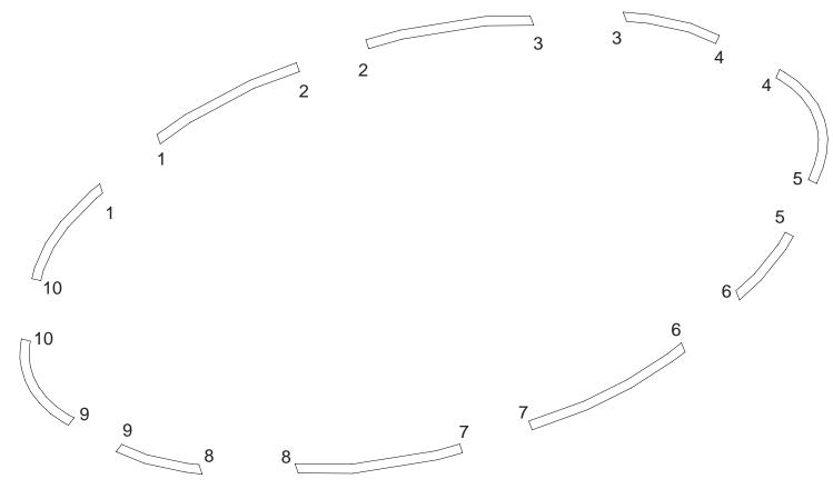
Assemble aero frame parts in numerical order.
